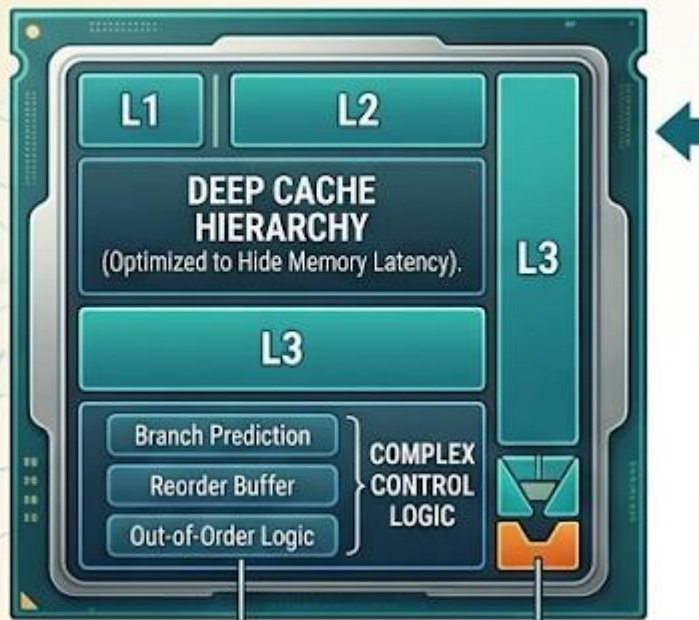
DEEP CACHE HIERARCHY (Optimized to Hide Memory Latency).
